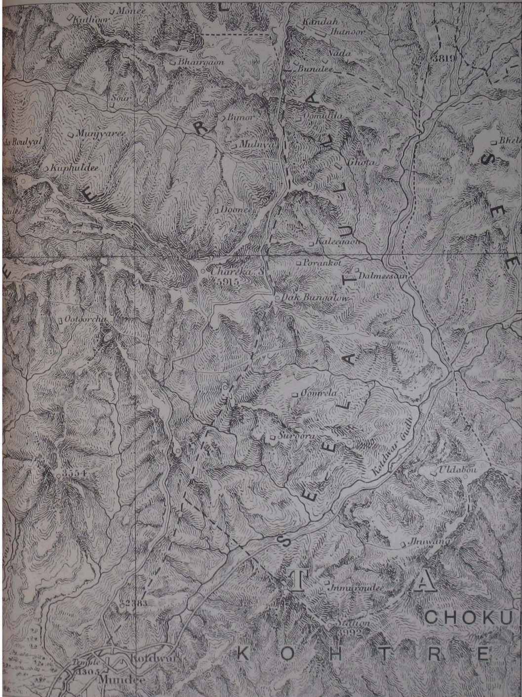
This sheet shows the old method of representing hills by horizontal hachuring, before the hachures had begun to approximate to form-lines or contours. The sheet was drawn on the scale of 1 inch to 1 mile for reproduction by photozincography.
