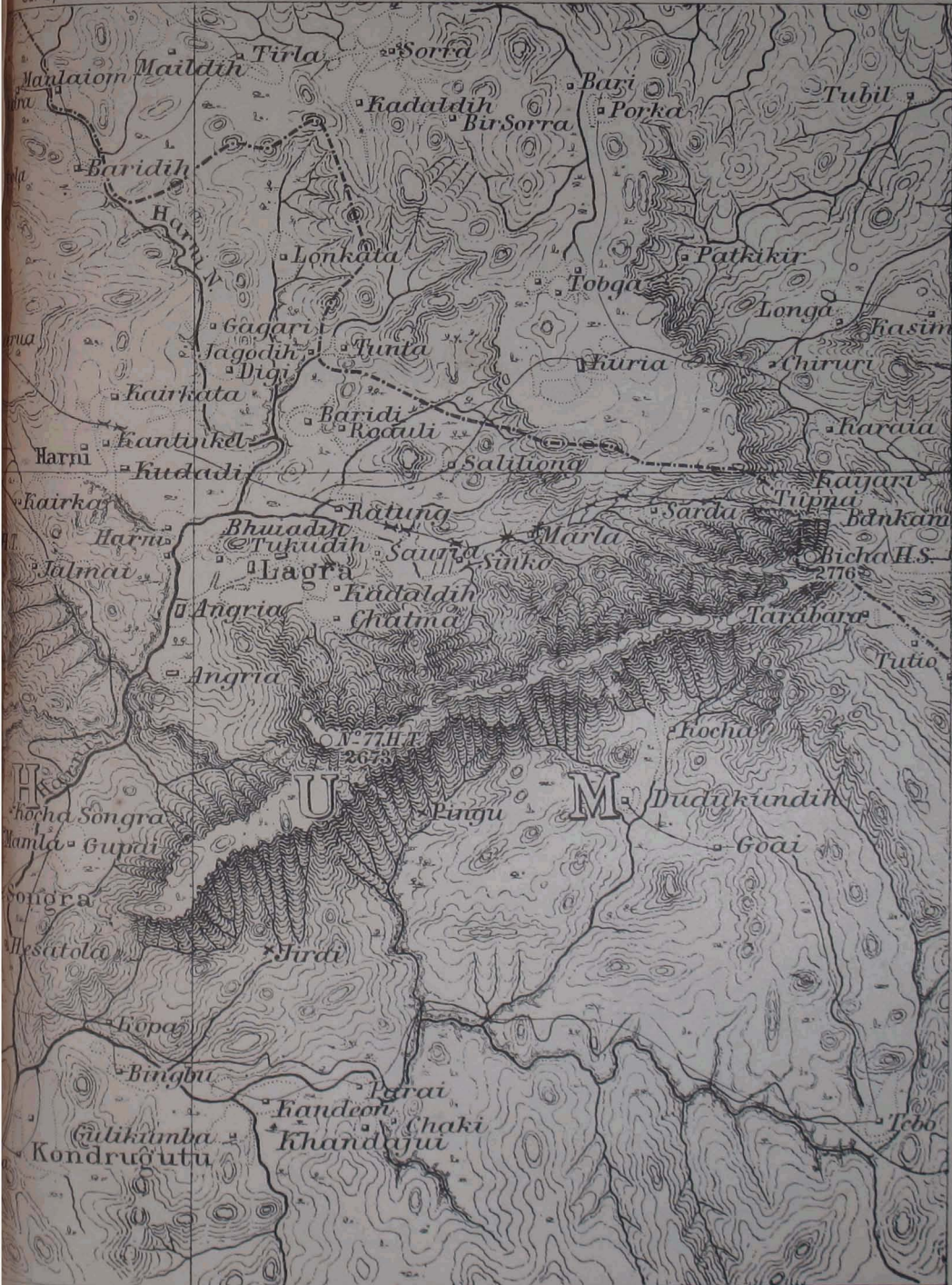
Surveyed and drawn on the one-inch scale and reproduced by photozincography. The approximation of the hachures to form lines may be noted.
